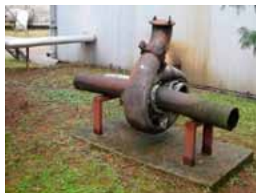
Pict. 10: Exhibit – pipe after explosion, in the oil refinery
